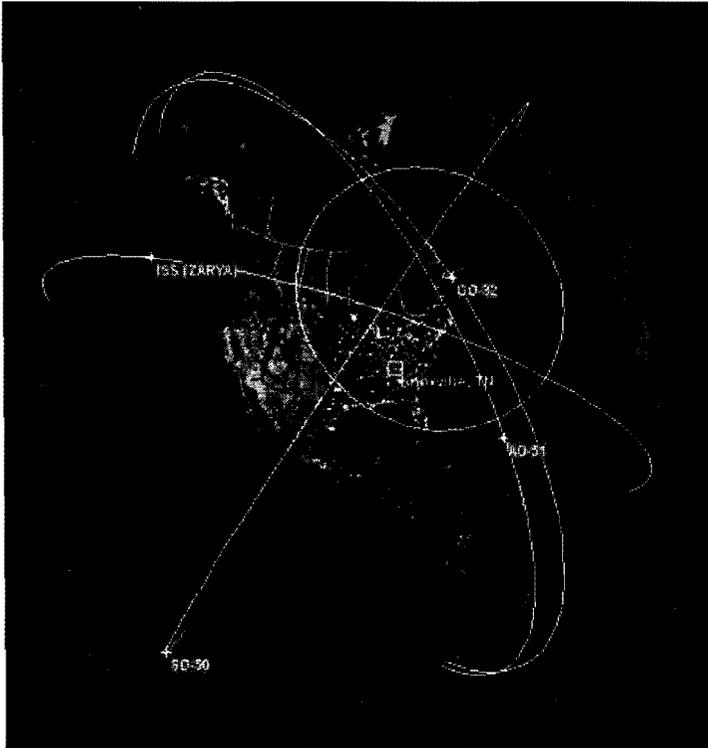
The sub satellite point (SSP) of AO-51 moves about 25° west each pass. At 39 °N latitude this is 1337 miles (2139 km). Mid-latitude locations will get a pass to the east and one to the west, and the second pass will be east, west or close to overhead. The more overhead the pass is (close to 90 °), the lower the first and third passes will be. AO-51 has a footprint of about 3900 miles in diameter; this will give all the mid-latitudes three passes in the morning and three passes in the evening.
