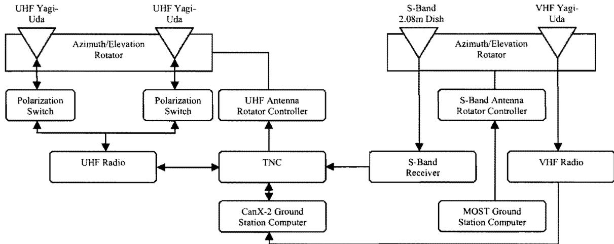
**Figure 2: Ground Station Architecture Diagram**
