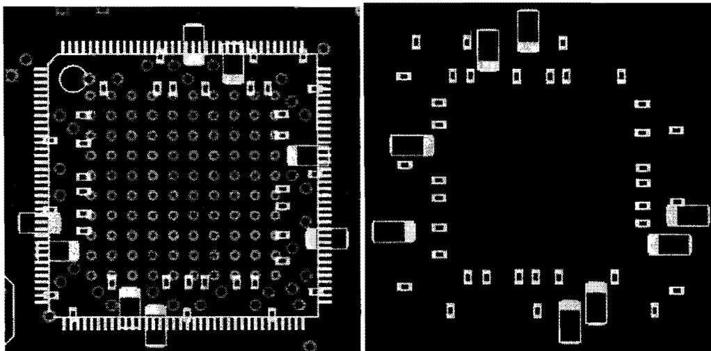
Figure 6 Layout of the PCB top and bottom, showing the thermal pads, ground power supply plane and underside mounted DSP decoupling capacitors
