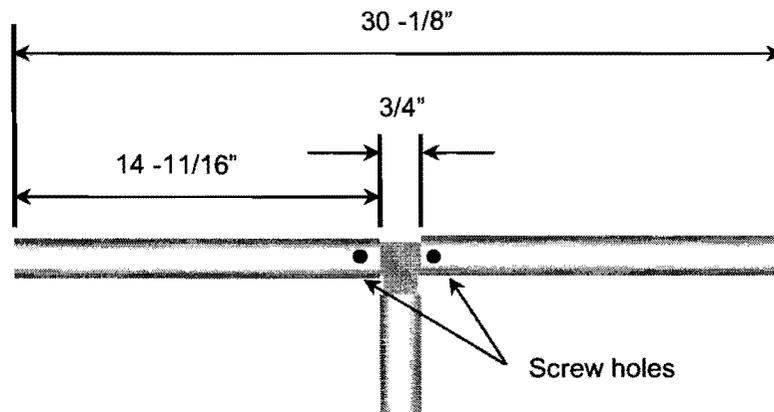
**Figure 6. Dipole dimensions**
