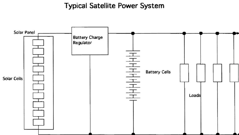
*Figure 1. Typical Satellite Power System*
