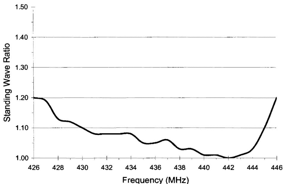
Figure 12. SWR versus frequency
