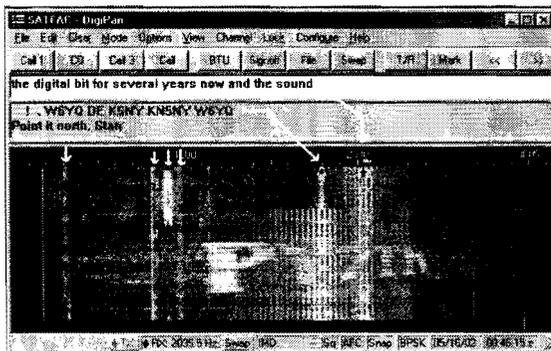
Figure 7. PSK-31 spectragram with 7 user signals.
