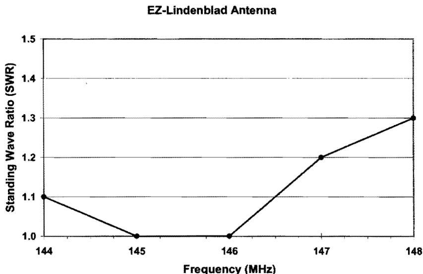
Figure 12. SWR versus frequency chart
