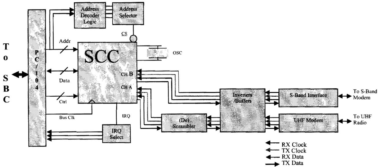
Figure 7: TNC Control Board Architecture
