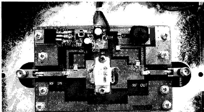
30W Amplifier Kit-  $V_{dd} = 28VDC$ , Gain=13dB,  $IDQ=360mA$ ,  $I_{max}=2A$ , Eff.=50%. Kit includes board and all components with the exception of the output/input connectors and heatsink. Shown is 5X7 inch sink with 24X1" fins. Base of fins can be seen through the milled holes under the SMA connectors.
