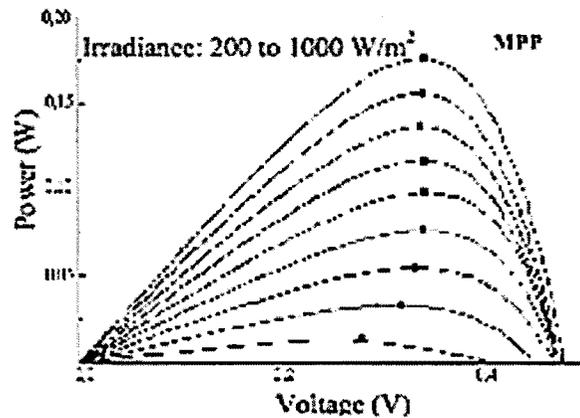
Figure 3 Typical MPP vs Irradiance curves
