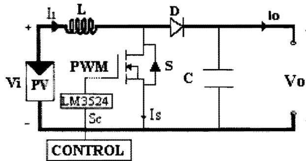
*Figure 4 Typical Boost Converter.*
