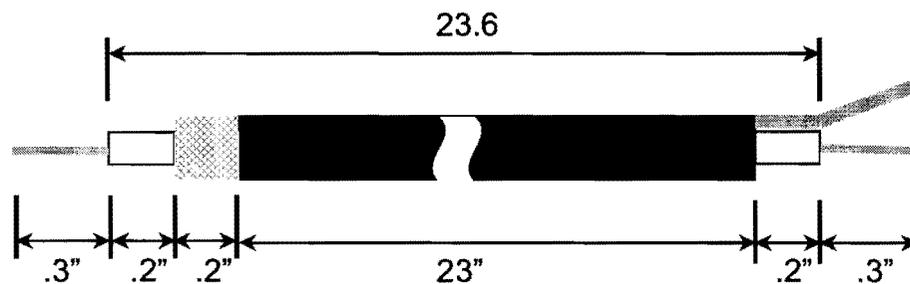
Figure 9. Coaxial feed cables
