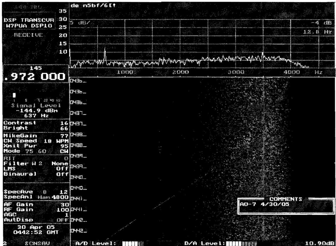
Figure 4 AMSAT-OSCAR 7 carrier trace, AOS through TCA.
