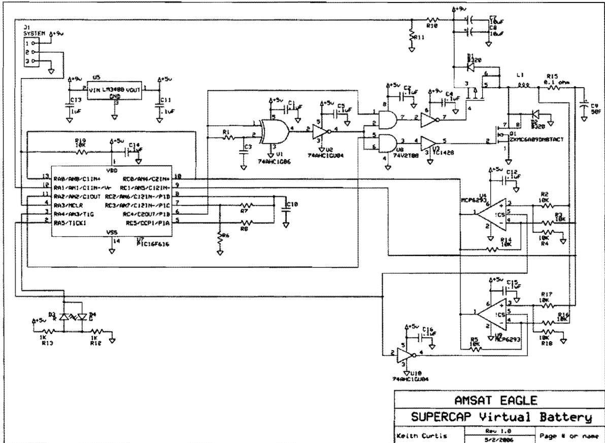
Figure 7 Super Capacitor Prototype Schematic
