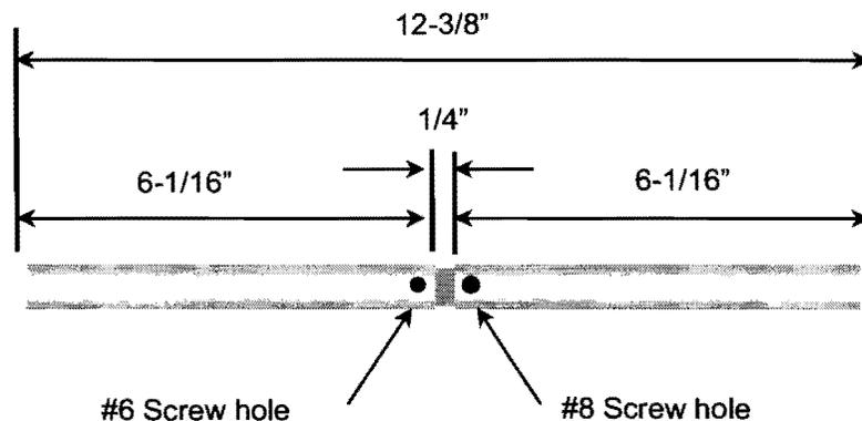
Figure 5. Driven dipole assembly
