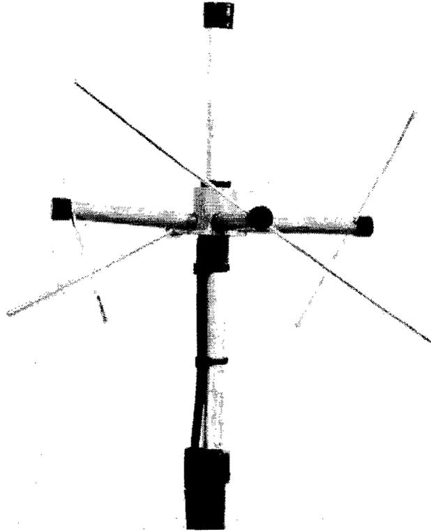
*Figure 9. The completed Parasitic Lindenblad antenna*
