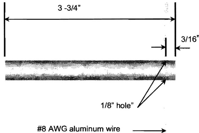
Figure 4. Parasitic element assembly
