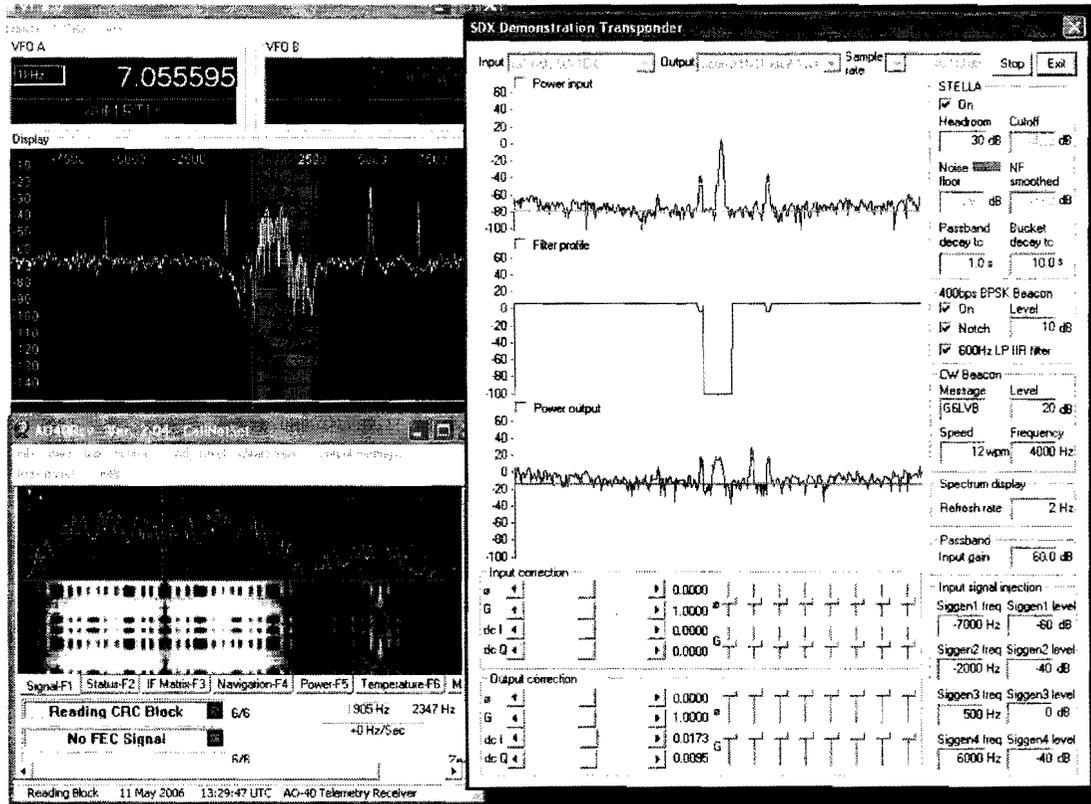
Figure 7 PC version of the transponder software showing telemetry decoding
