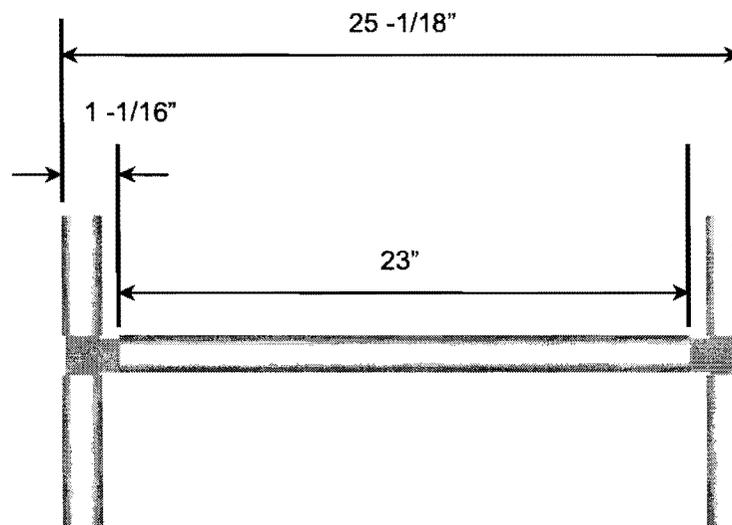
**Figure 7. Cross-boom assembly dimensions**
