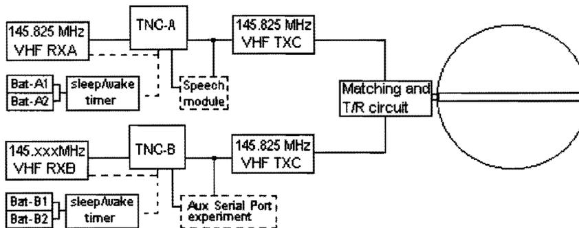
**RF System:** ANDE has two independent AX.25 Packet Command and Telemetry systems. The primary system operates like PCsat providing Telemetry on 145.825 and supporting users communications. The secondary is on unpublished frequencies.
