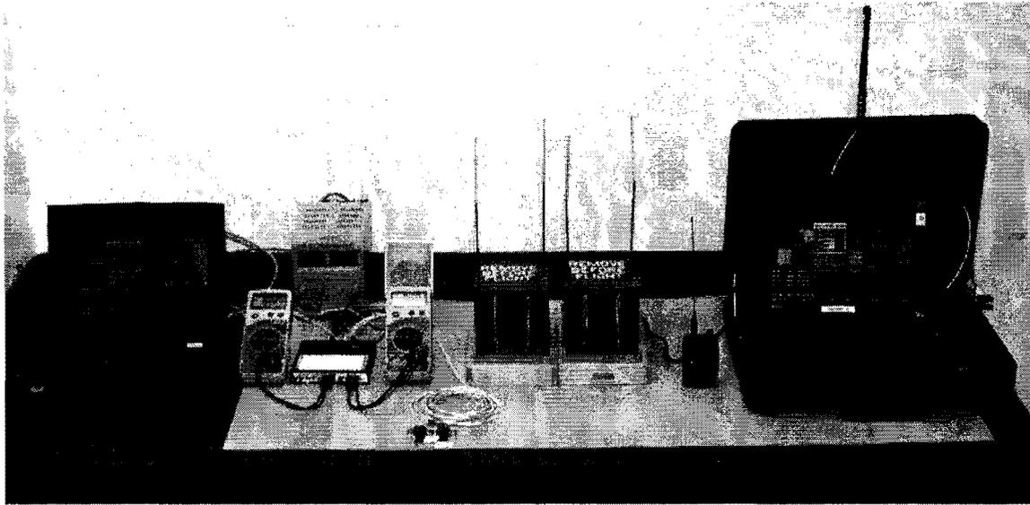
The photo above shows the RAFT and MARScm pair as they were delivered for integration and checkout. The laptop on the left connects via the umbilical for testing and the briefcase on the right is the complete RF ground station using a laptop and a TH-D7 APRS radio for the comms link. Each satellite not only has a pair of VHF spring loaded whip antennas to help separate them, but also a 4 foot deployable HF antenna.
