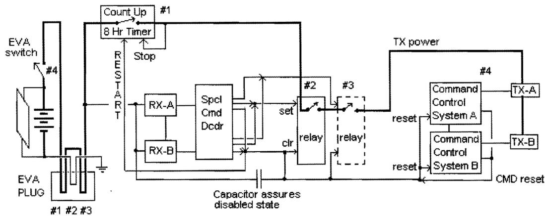
Figure 6. PCSAT2 Multiple transmit inhibits required for Astronaut Safety during EVA.
