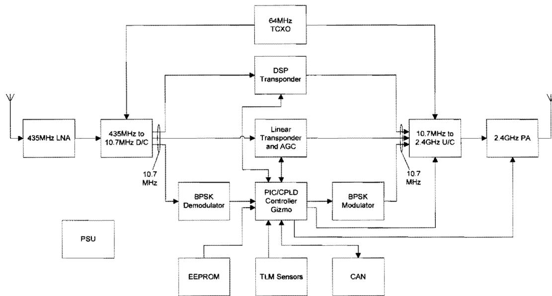
Figure 1 The AMSAT-UK ESEO payload
