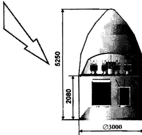
Standard Dnepr-1 Space Head Module configuration is arranged in double tiers, which enables multiple small spacecraft deployment capability (up to 10-15 small spacecraft).
