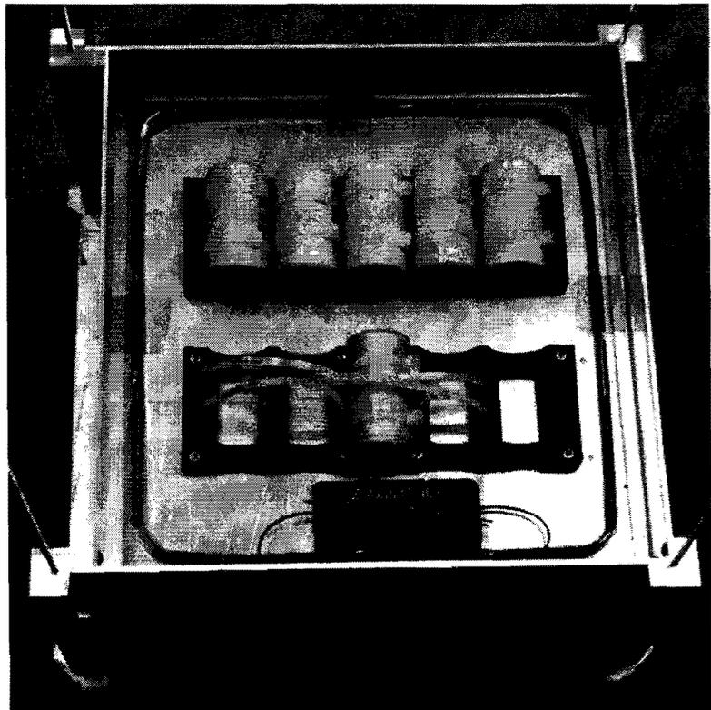
Photo shows sample cells and battery holder with the Z axis coil.
