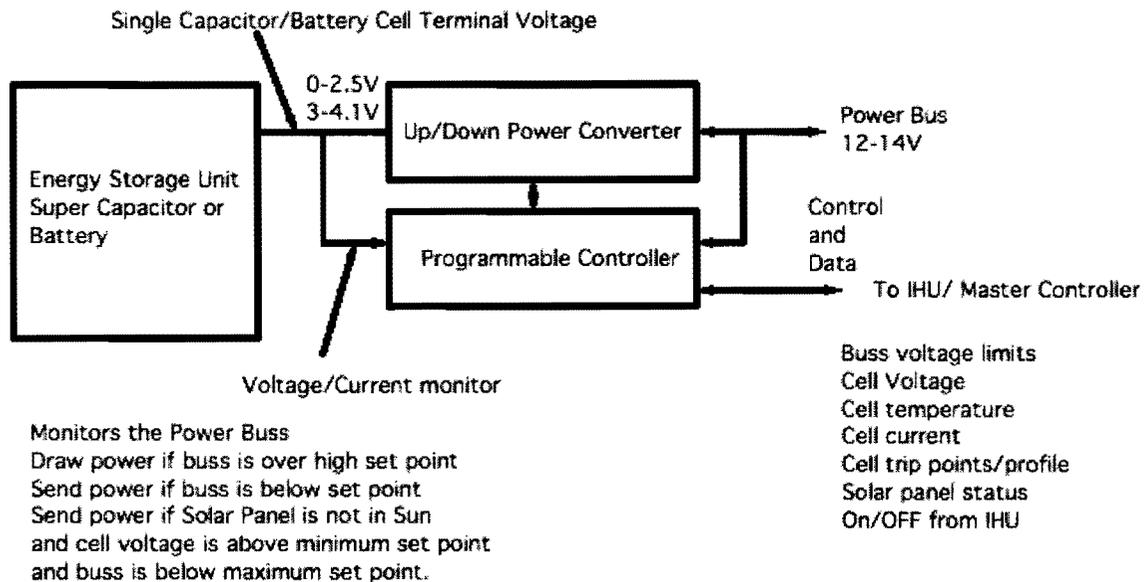
Figure 6 Virtual Battery System
