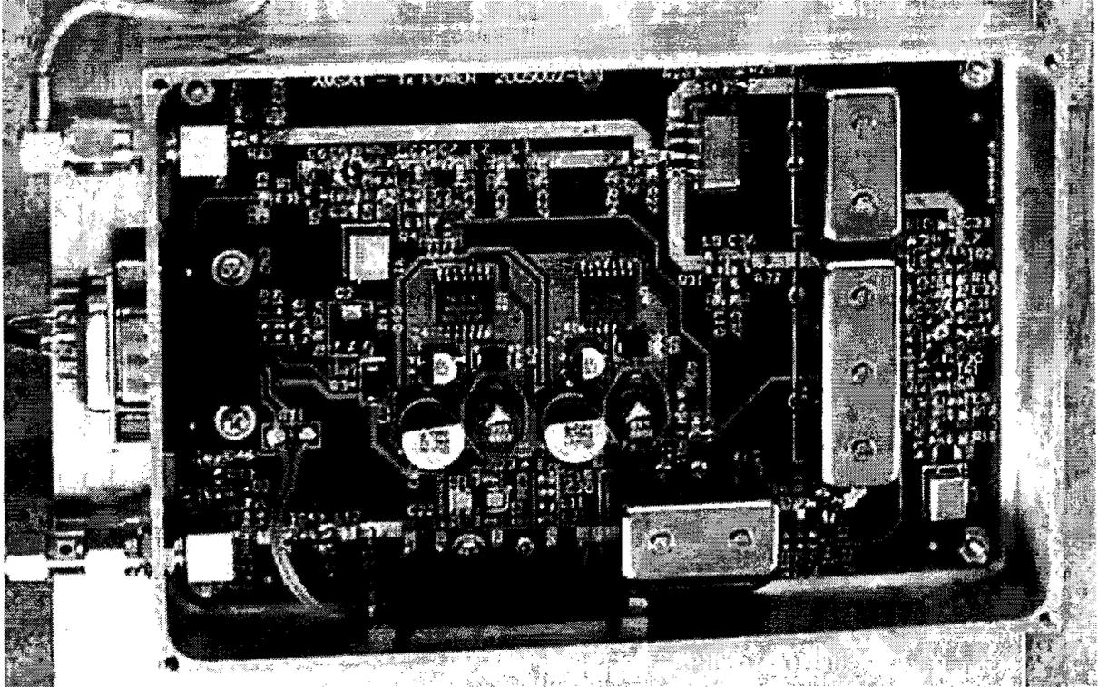
Linear VHF 2 Watt PEP transmitter – (30 kHz bandwidth) (ZL2BAC)
