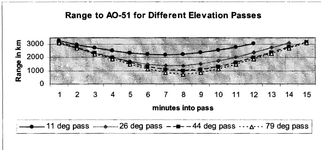
Figure 6, Distances to AO-51 at selected Maximum Elevations
