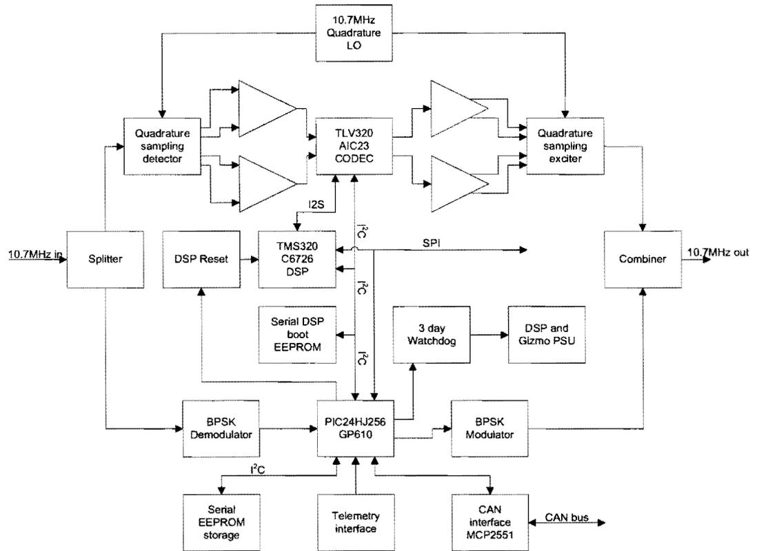
Figure 2 AMSAT-UK's ESEO payload: DSP and control system
