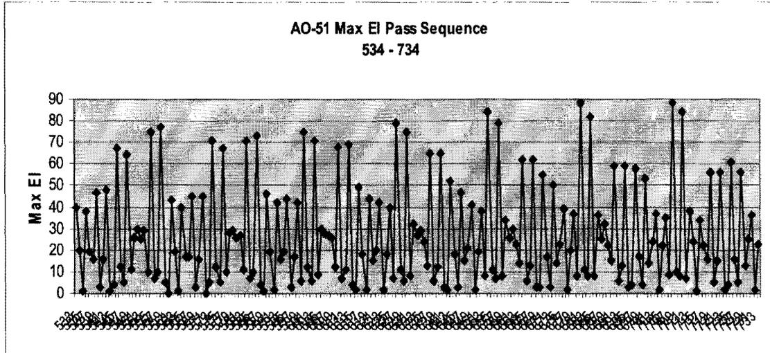
Figure 10. Typical AO-51 pass sequence at EM75xw showing 200 passes
