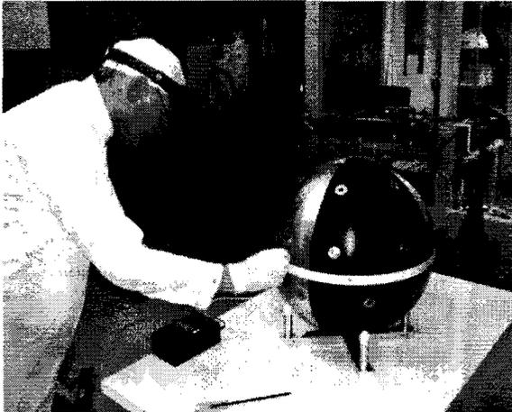
This photo shows the final SWR tweaks to bring the hemispheres into resonance. The antenna actually is more of a slot antenna formed by making 18 of the 36 bolts that connect the two halves be conducting and 18 of them being insulating and feeding the insulated half in the middle.
