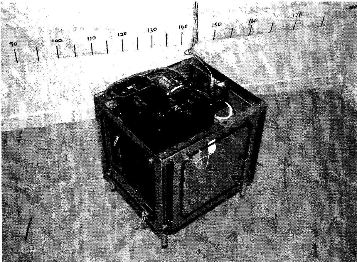
Single axis Attitude Control test rig with Magnetometer
