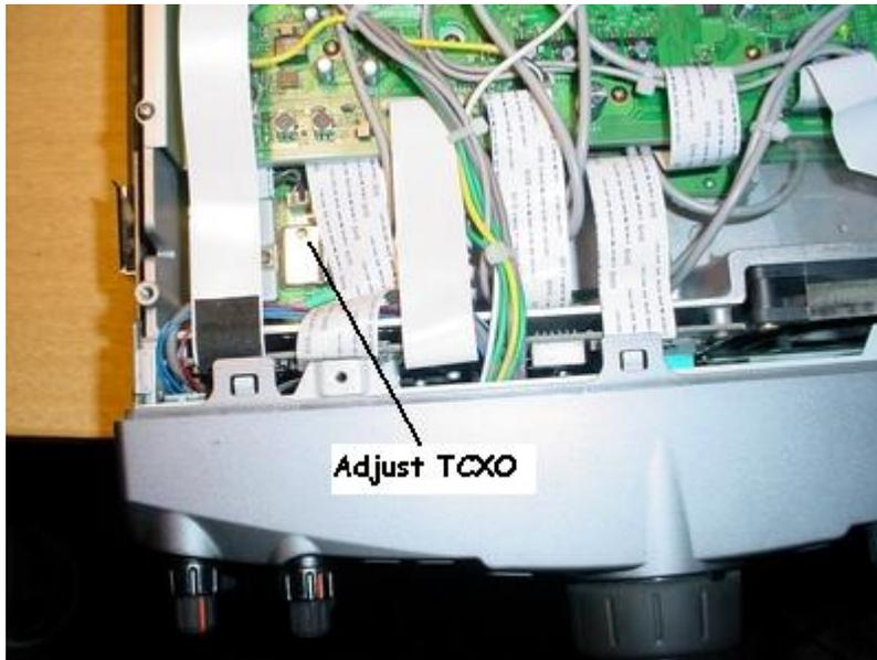
The master oscillator adjustment can be accessed from the bottom. Turn the radio upside down and remove the bottom cover. The photos show the oscillator adjustment point.
