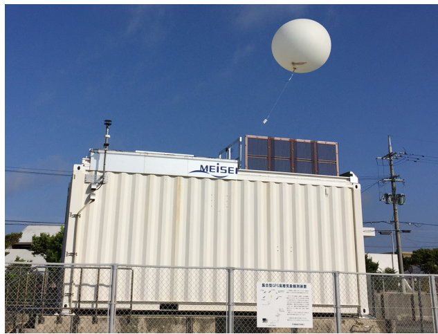
ABL: Automatic Balloon Launcher
