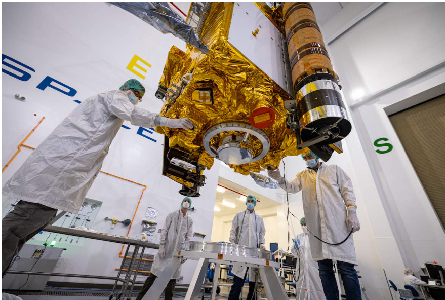
NASA's DART spacecraft during pre-launch processing at Vandenberg Space Force Base, California. One of the spacecraft's roll-out solar arrays is visible on the right. Credit: NASA/Johns Hopkins APL/Ed Whitman
